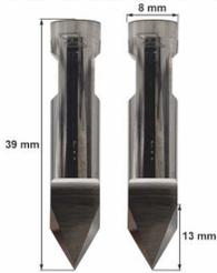
**Description:** Knife blade with 8mm cylindrical shaft for use with the RM (RigidMaterial) knife tool. 2 times 30 degrees angle. Can cut up to about 5-6mm thick materials.
