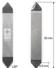
**Description:** Centric, asymmetrical drag knife for ridge-free inside cutting edge. Equivalent to the Z10 / HTZ-012, but with the part of the cutting edge lowered to 0.63 mm.
